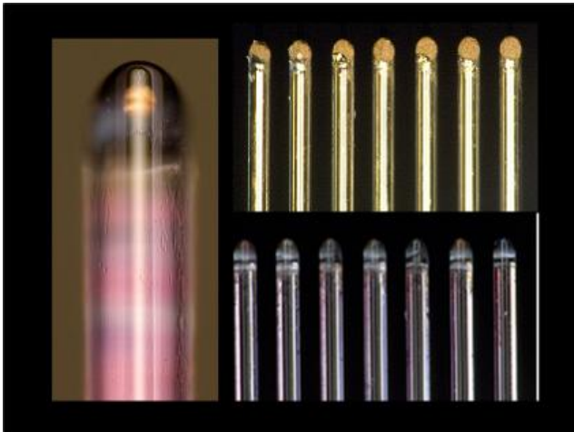
Figure 9. Left is close up of fiber end showing emitted light. Top is underside of fiber with reflective coating. Bottom is top of angle cleaved fibers.
