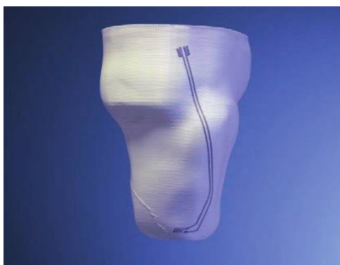
Fig. 12 | Leg prosthesis part produced by FDM and Aerosol Jet printing. Figure reproduced from ref. 31 , University of Applied Science Bremerhaven.
