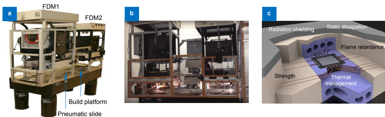
Fig. 1 | (a, b) Photograph of the multi 3D system. (c) Schematic of a fabrication example. Figure reproduced from: (a) ref. 9 , Springer International Publishing AG; (b) ref. 14 , Elsevier Ltd; (c) ref. 9 , Springer International Publishing AG.
