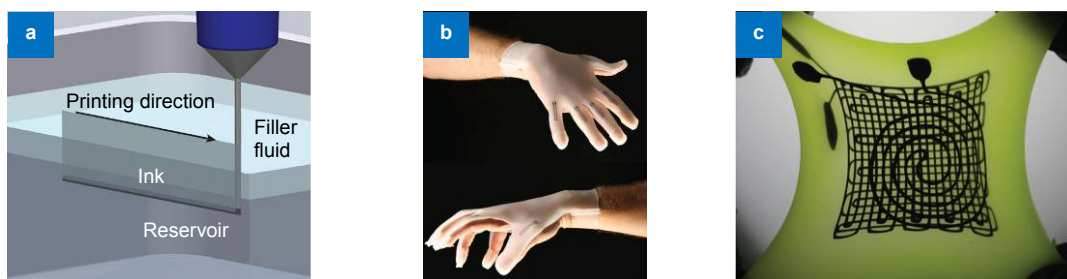
Fig. 9 | Schematic illustration of the embedded 3D printing (e-3DP) process and printed stretchable electronics. (a) Schematic illustration of the e-3DP process. (b) Photograph of a glove with embedded strain sensors produced by e-3DP. (c) Photograph of a three-layer strain and pressure sensor in the stretched state. Figure reproduced from ref. 11 , WILEY-VCH Verlag GmbH & Co. KGaA, Weinheim.
