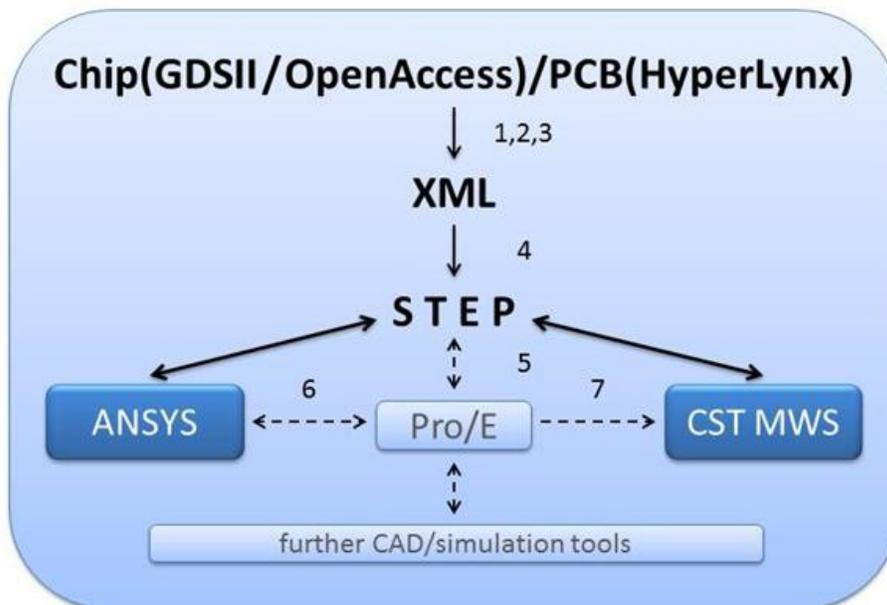
Figure 3 Converting the XML based description to standard FEM tools
